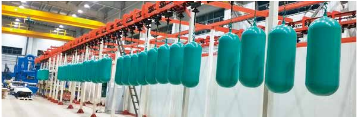
钢质无缝气瓶生产五车间喷涂工序
